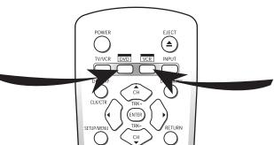
**VCR Button** - Press to control the VCR deck. All deck control keys and red labeled buttons will operate the VCR.
